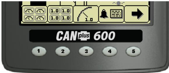
Five buttons access a context dependent **button bar** when any button from 1 to 4 is pressed. The graphical menu structure uses easily understood icons to indicate the button's current function. After 5 seconds of inactivity the button bar disappears.
